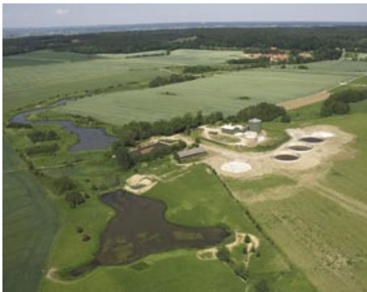
The Wrams Gunnarstorp estate may be viewed as a model on the path to a sustainable agriculture and food-processing industry in Sweden. The facility processes waste from hog farming using an almost odorless process. Biogas is extracted from the waste, and this can be used to replace energy and thus reduce carbon dioxide emissions, in addition to nitrogen and phosphorus, which are returned to the soil in the form of fertilizer.
