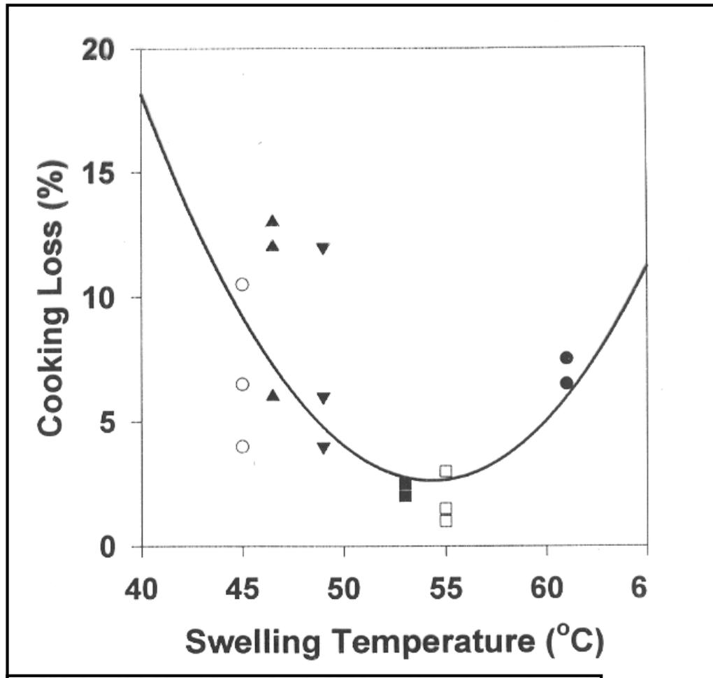
Cooking losses in sausage batters when heated to 75°C, as a function of the starting temperature for gelatinization (judged using light microscopy) of different starches: (2:□) native potato starch, modified potato starches (3:▼, 4:▲ and 5:○) and amylopectin starches from barley (6:●) and potato (7:■). ( $r=0.67^{**}$ )
