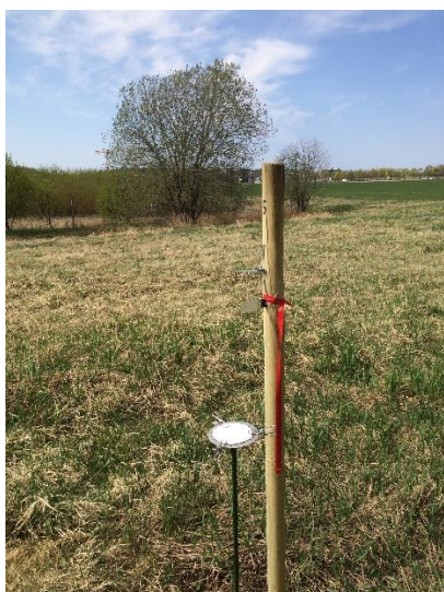
Figure 2. Spore traps from Ultuna, Uppsala, Sweden, in 2019.
