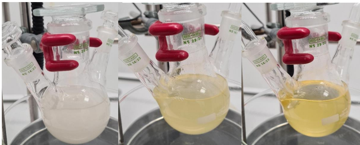
Figure 3. Dissolution of cellulose in DMSO with DBU and CO 2 . On the left before bubbling of CO 2 , in the middle after 30 min and on the right after 4 h, when the reaction was complete.
