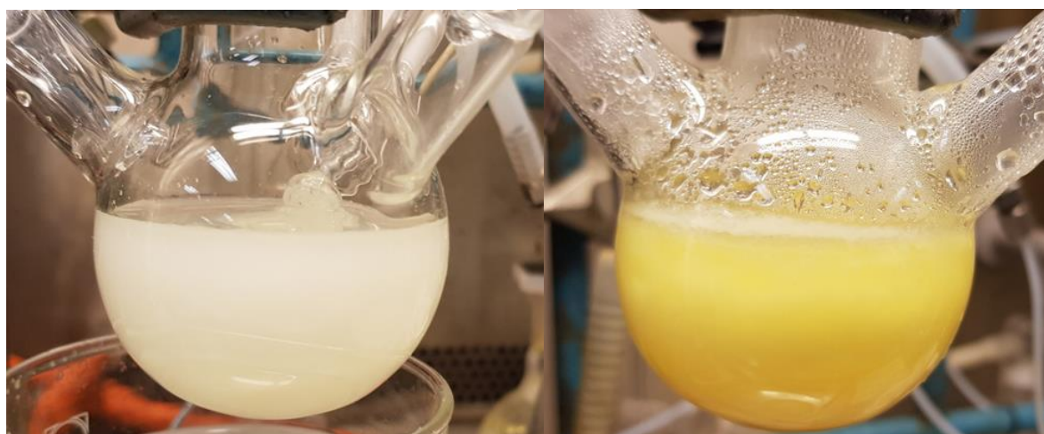
Figure 2. Cellulose dissolution experiment with PEHA and CO 2 in DMSO. On the left before bubbling of CO 2 and heating. On the right after the reaction.
