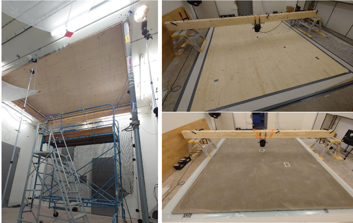
Figure 2. Left photo show the receiving room (at RISE building acoustic laboratory in Borås, for impact sound measurements of floors), where the test CLT floor is rigged with 5 x 5 accelerometers on its ceiling. Some of the microphones are also seen in the photo. The photos on the right show the above side of the floor, where the excitations and force measurements were made. The upper right shows the bare CLT- slab and the lower right shows the floor with a heavy floating screed above an impact sound insulation layer on top the CLT slab.
