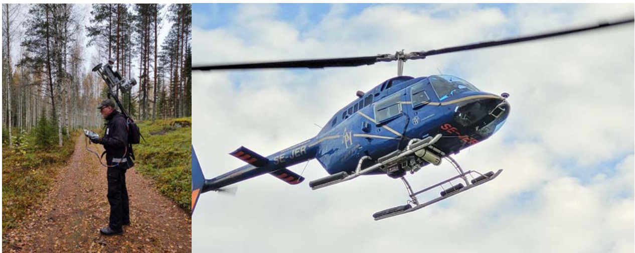
Figure 1. a) Akhka-R4DW backpack dual-wavelength (905 nm + 1550 nm) laser scanning system, and b) three wavelength (532 nm + 905 nm + 1550 nm) helicopter scanning system was developed in the project and used for forest plot surveys, here in October 2021 in Hällefors region, Sweden.
