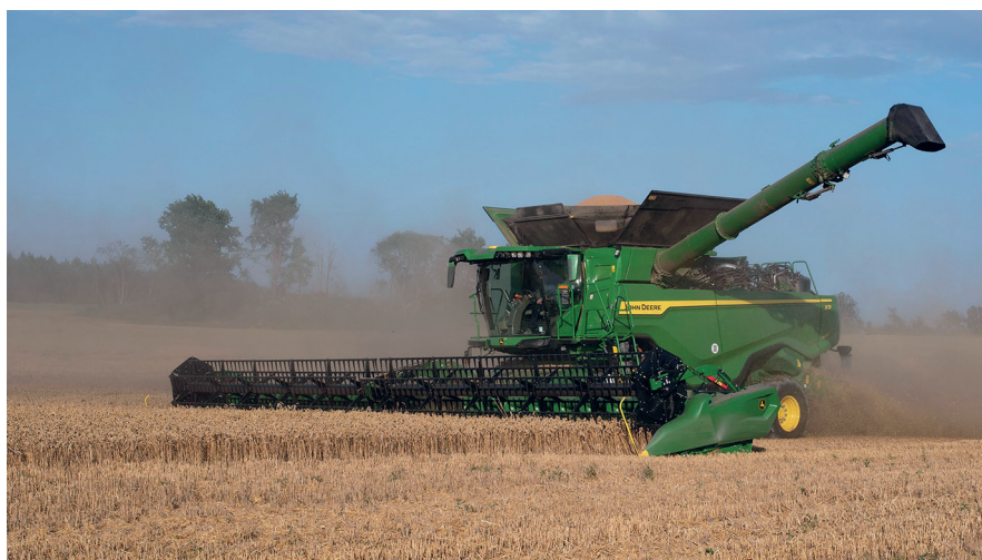
Figure 1. This X9 combine from John Deere can harvest 100 tons per hour. Photo: Per Frankelius.
